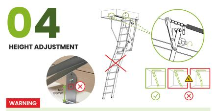
The ladder cannot be moved to the mounting hole marked in red, as the distance between the centre of the rung and the trapdoor must be greater than or equal to 100mm.
